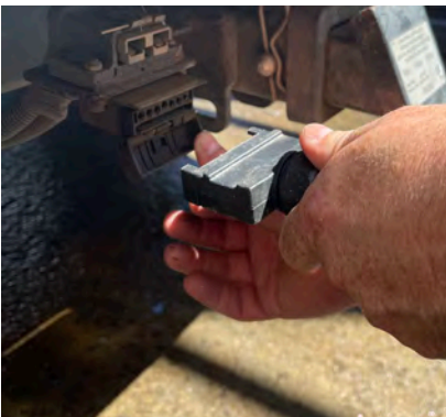
5. Plug in the Anderson plug into rear of vehicle
