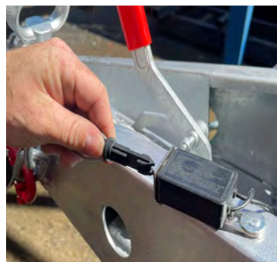
8. Plug breakaway switch back into unit
