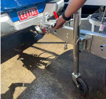
1. Reverse vehicle so tow ball is under hitch. Wind Jockey wheel down
