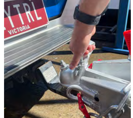
3. Wind jockey wheel down onto tow ball and ensure hitch lock is down
