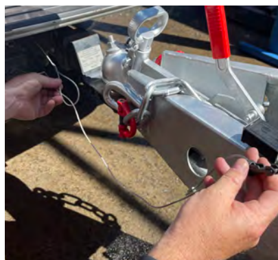
7. Remove breakaway switch from unit and wrap cord around tow bar
