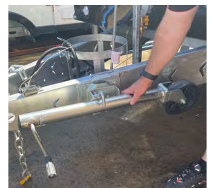
9. Wind up jockey wheel, pull handle and lock into place
