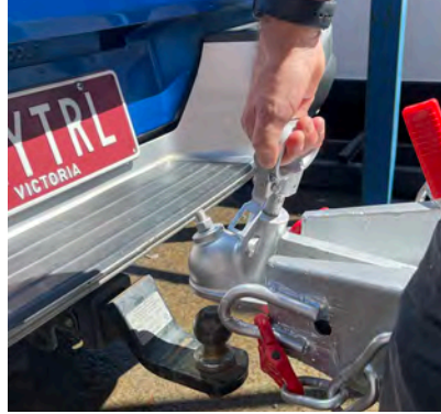
2. Ensure hitch lock is lifted up
