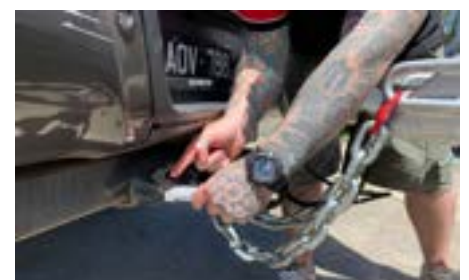
Disconnect your trailer plug & any other elec. connections to the trailer
