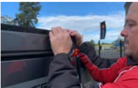
Release the over-centre catches
