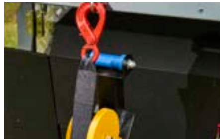
The winch should lock into position like this
