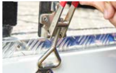
Release the over-centre latches
