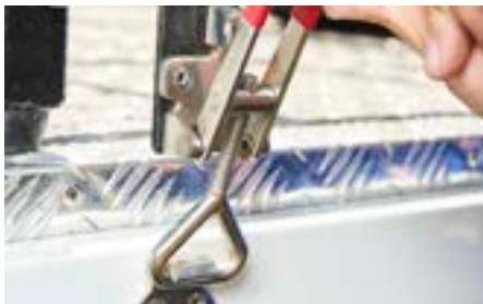
Release the over-centre latches
