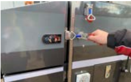
Unlock the the latches at the side of the camper
