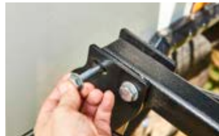
Remove the locking pin on the other side of the trailer
