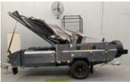
Then use the rear winch to safely lower the lid into position
