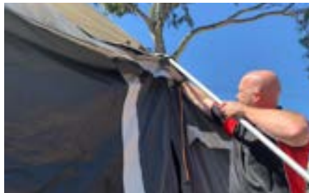
Insert the hooked end of the pole through the loops on each tent bow
