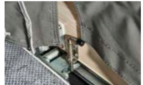
The locking pin needs to be released inside before sliding the bed out
