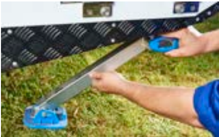
Lower all legs into position & Use your winder tool to stabilise the trailer
