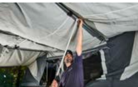
C-clip spreader bars stop water from pooling in bad weather
