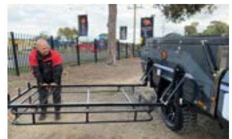
Or it can be locked vertically (Replace the bolts to lock in the rack)
