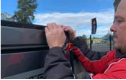
Release the over-centre catches
