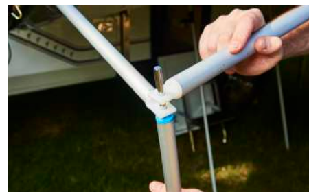
Upright pole, followed by the ridge pole, then the flat end spreader bar.
