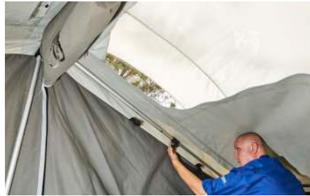
Attach the longer c-clip spreader bar
