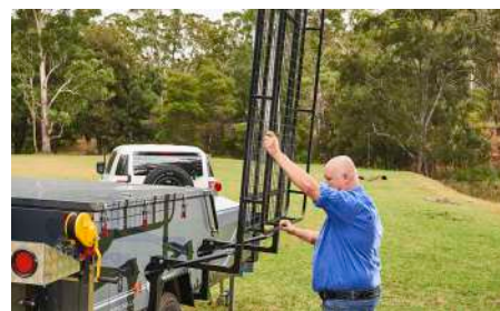
Or it can be locked vertically (Replace the bolts to lock in the rack)
