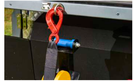
The winch should lock into position like this
