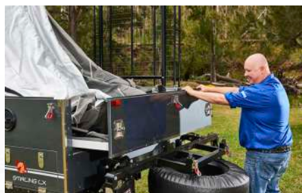
Slide your rear bed out after unlocking the latches and the pin inside
