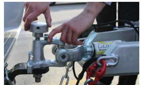
Take off hitch lock, push pin to the outside and unscrew the hitch bolt
