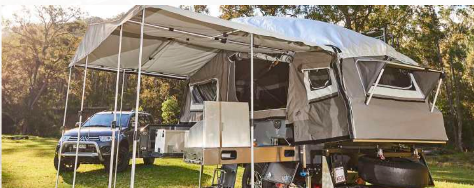
C-clip spreader bars stop water from pooling in bad weather
