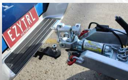
Flip the hitch over to clear space to drive vehicle away
