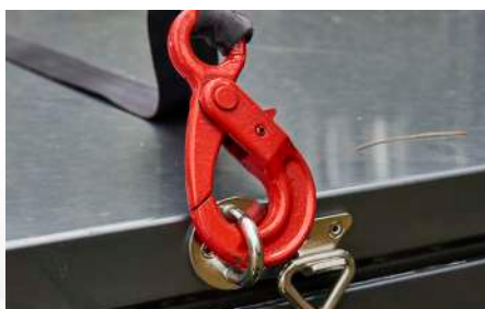
Attach hooks to the anchor points
