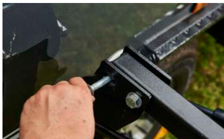
Remove the locking bolts on the other side of the trailer
