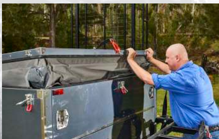
Lift the lid around 500mm or so before winching
