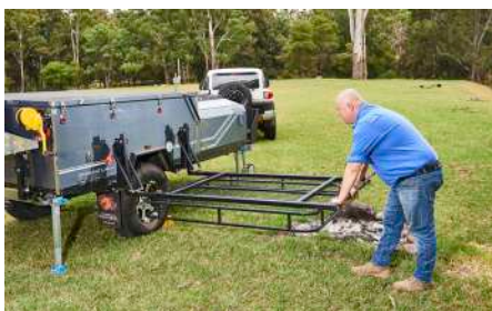
The rack can be locked horizontally (Replace the bolts to lock in the rack)
