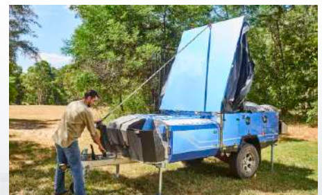
Use the front winch to get the lid past 90 degrees
