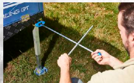
Lower all legs into position & Use your winder tool to level the trailer
