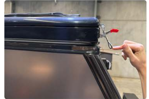
3. Place D-latch pin back through guides and sit roof latches in - to ensure it doesn't get in way of roof
