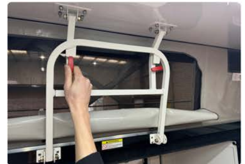
6. Once lifting bar locked in place - ensure red latches are turned to hold bar in place
