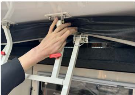
4. Remove the D-latch pins holding the roof lifting handle in place from both left and right sides
