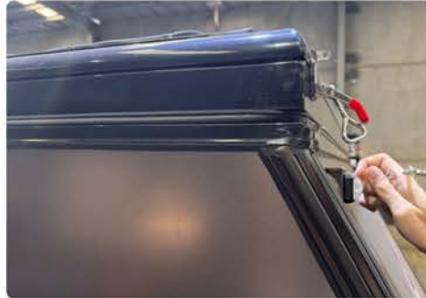
2. Unclip the roof latches on all 4 corners of roof
