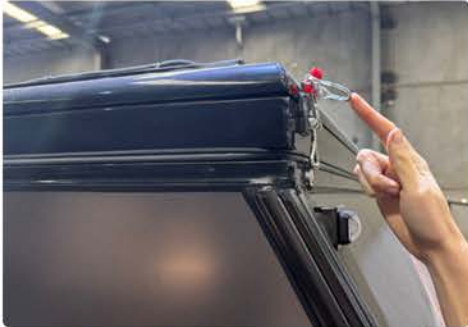
1. Unclip the D-latch pins on all 4 corners of roof
