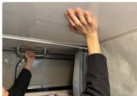
8. Move to opposite side of van, one hand on roof and other on handle to raise the roof in place.
