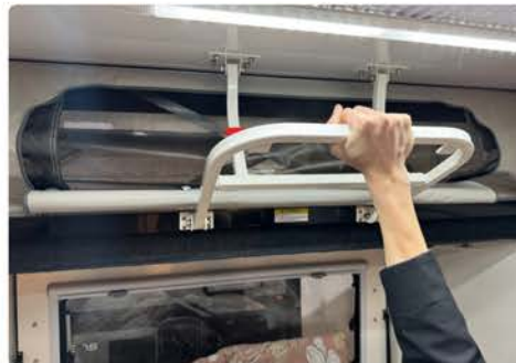
5. Grab the bottom bar and lift the handle. Continue lifting until the bottom bar touches the bars holding on to the roof
