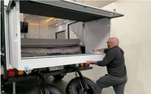
9. Grab the handles on the back window panel and raise it into the upright position
