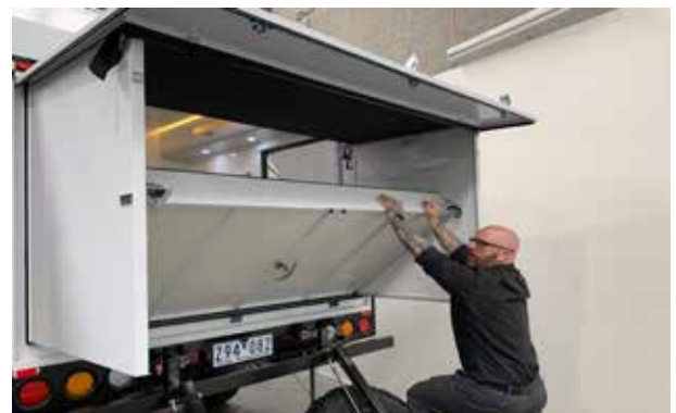
7. Raise the bed, returning it back to its travelling position
