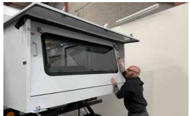
4. In the upright position, make sure to unclutch the slide bolts onto the side walls
