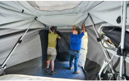
Swing the bow out and up and once extended, lock it into position
