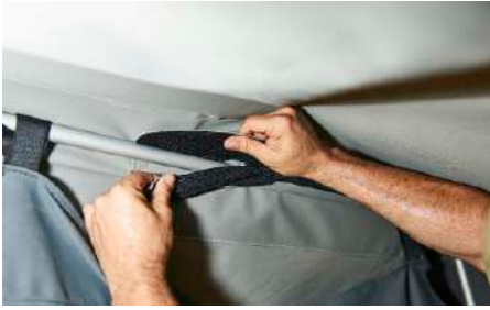
Use the Velcro to attach the roof bow to the roof
