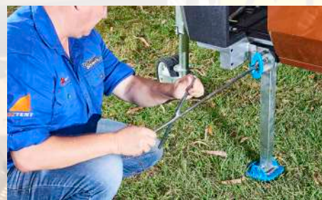
Lower all legs into position & Use your winder tool to level the trailer
