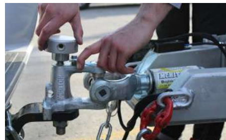
Take off hitch lock, push pin to the outside and unscrew the hitch bolt
