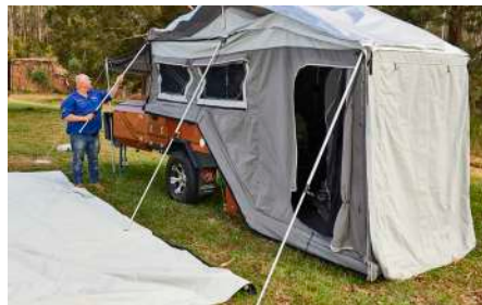
Ridge poles in position and ready to go, with the centre tent bow lowered for easier access
