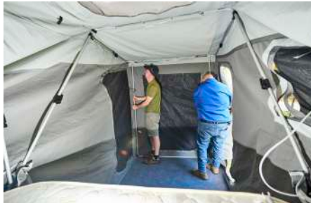
The C-Clip uprights need to be in to hold the bow in position
